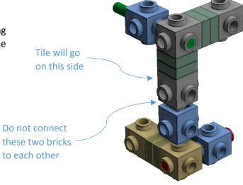
Connect the tile to the edge assembly to lock its correct length.
