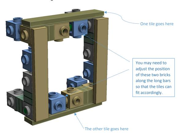
Repeat step 9 with the other two remaining edge assemblies from step 8.
