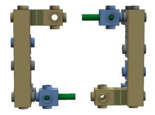
Connect the two edge assemblies through their long bars only so that you can also connect the tiles to the newly created edges and lock their correct lengths.
