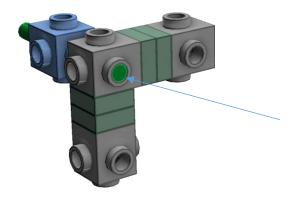
Make sure the end of the long bar stays aligned with the top of the stud (flushed)
